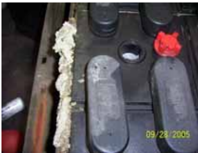
White deposit is growing on cel 16 & 17. (Showing physical damage.)
